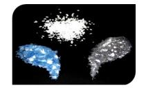
Vinyl chips produced from rigid vinyl film via the calendaring process are grinded and sieved to the size chose by our clients. All of our production is based in our French factory and can be formulated with low phthalates components below the JT reference (toys standard, EN71-3, EN71-2: 1994).
